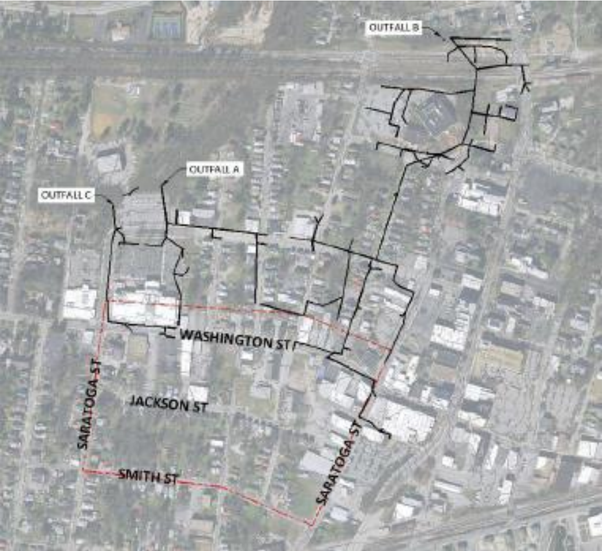
Existing Storm Sewer Network
